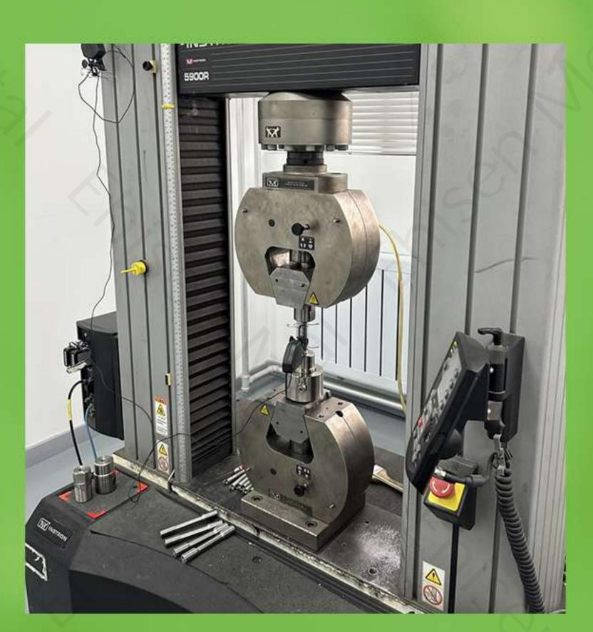
NORMAL TEMPERATURE TENSILE TESTING MACHINE
